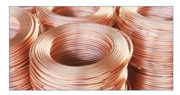
Pancake coil is the most popular form for delivery, it has a smooth, clean and dry inner surface, and manufactured in accordance with ASTM B 280 or EN 12735-1. Made of Cu-DHP, soft annealed and in the package of cardboard boxes with shrinking PE bag.
