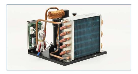
The direct current condensing unit for 12V /24V / 48V DC power supply can be used in mobile cooling systems with refrigerant R134a.
